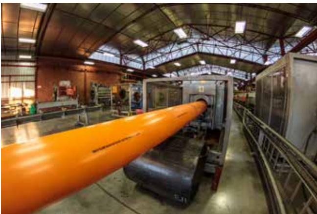
FIGURE 3.12A: EXTRUSION OF AN HDPE GAS PIPE
