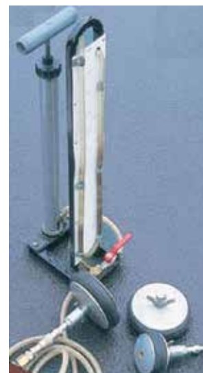
FIGURE 4.23: AIR TESTING EQUIPMENT
