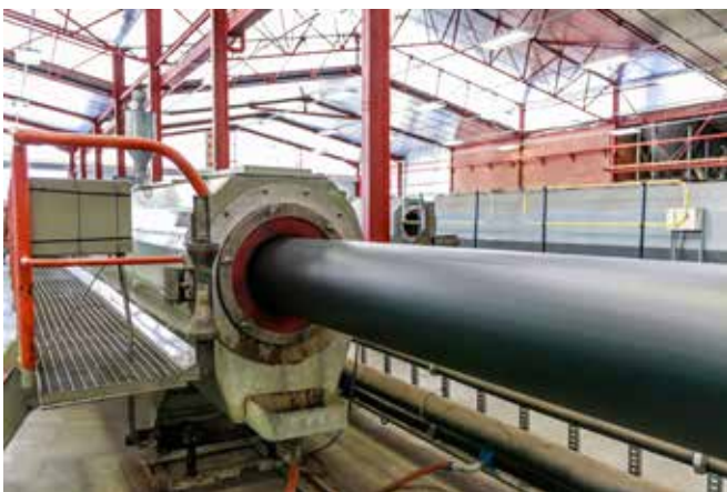
FIGURE 3.12B: EXTRUSION OF AN HDPE PIPE
